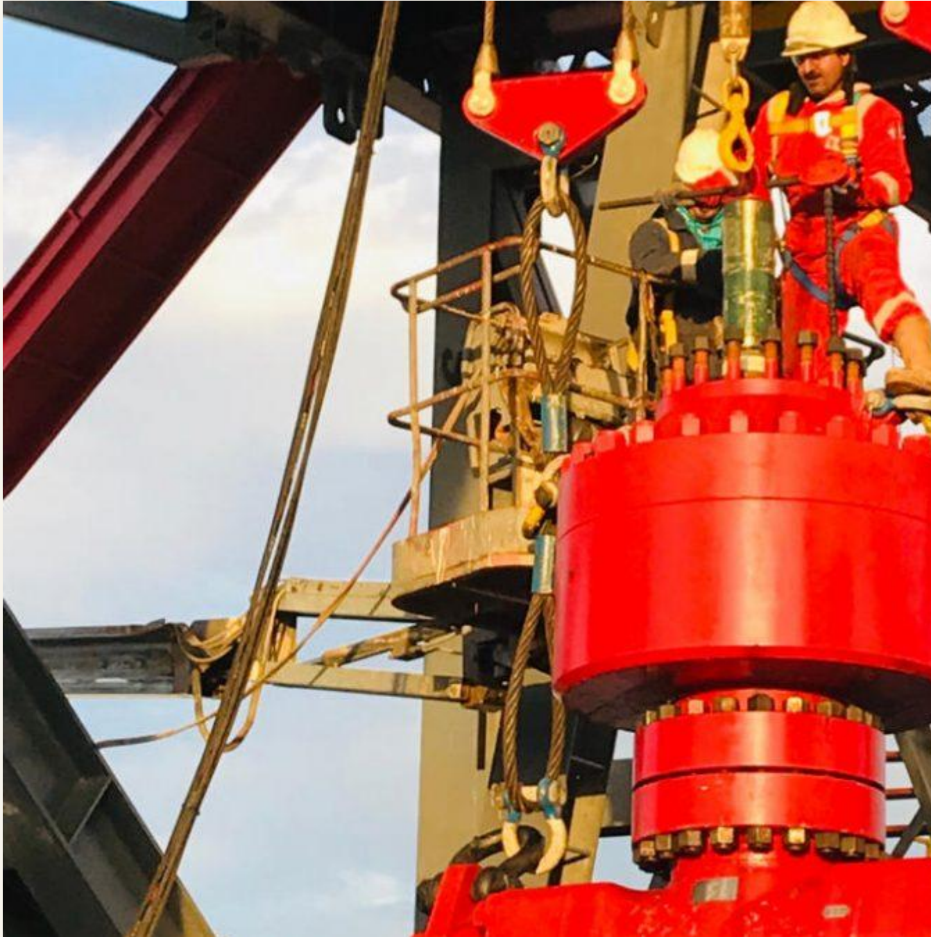
Blowout preventer (BOP) operations: the emergency mechanical barrier at the end of a long chain of protection.
